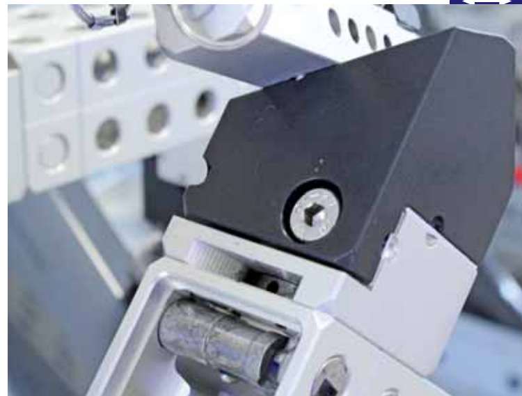
Application example: Clamping unit with ratchet clamp mounted on machined contour block (green) with 3D shim block base
